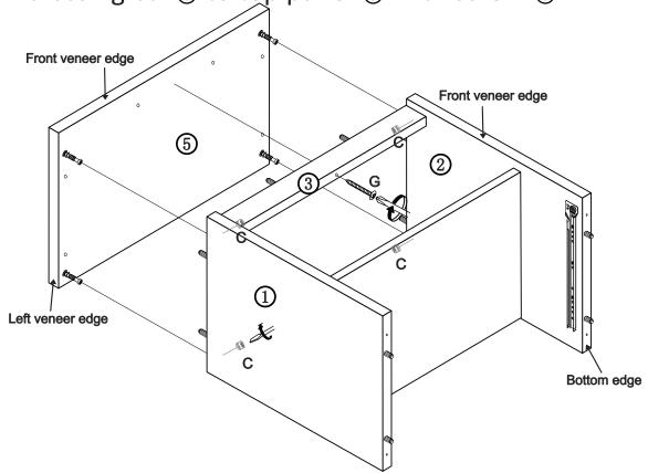
STEP 6: Attach bottom panel @ onto existing unit with screws ® .
