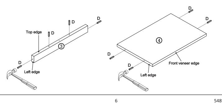
STEP 3: Attach crossing bar ③ and shelf ④ to left side panel ④ and right side panel ② with the dowel.
