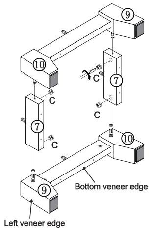
STEP 10: Attach the bottom parts to existing unit with screws © .
