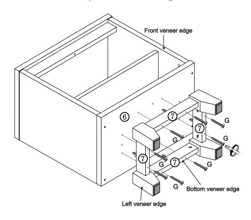
STEP 11: Attach back panel @ onto existing unit with screws ® .
